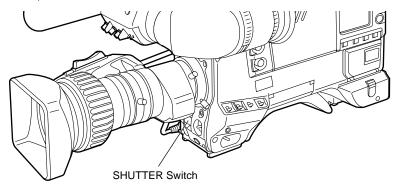
Press the SHUTTER switch to the SEL side repeatedly until the desired mode or speed appears. When all modes and speeds can be displayed, the display changes in the order shown below. If the required shutter speeds and modes have been designated beforehand, only the designated speeds or modes appear.
